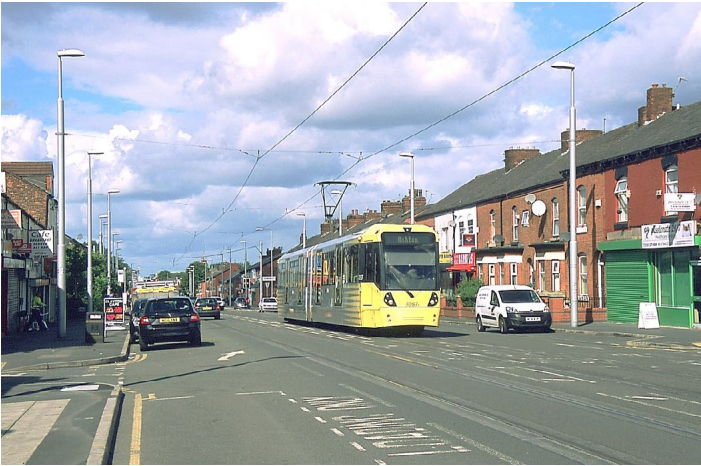
An outbound tram approaches the Edge Lane stop on Manchester Road. A substantial portion of line 3 consists of street operation with the trams mingling with motor traffic. In other locations, where the street is too narrow to host a stop, the tracks are routed off the roadway to stations alongside.
