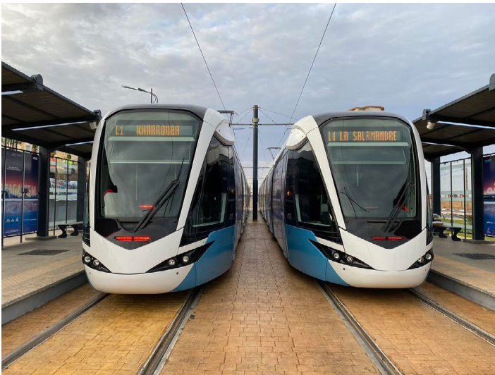
The new Mostaganem light rail system uses Citadis LRVs manufactured at the Cital plant in Annaba, northeast Algeria. Alstom photo
