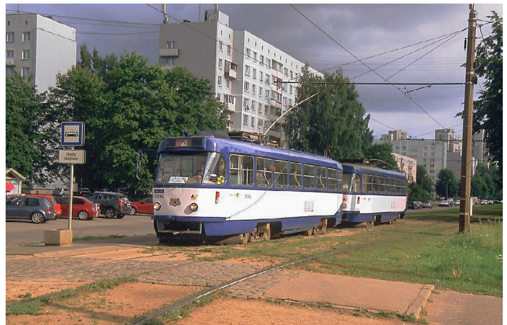
This train of Tatra T3s goes back to 1981 and is representative of the majority of cars operating on Riga's tramway system, all with trolley poles. The location is the Imantas iela stop along Bebru iela, a wide suburban-like arterial with a grassed center reservation. There are 134 of these fine PCCs on the roster. At the time of my visit route number 4 was assigned to tripper cars that beefed up rush hour service on the western end of route 1, but this route designation is no longer used.
