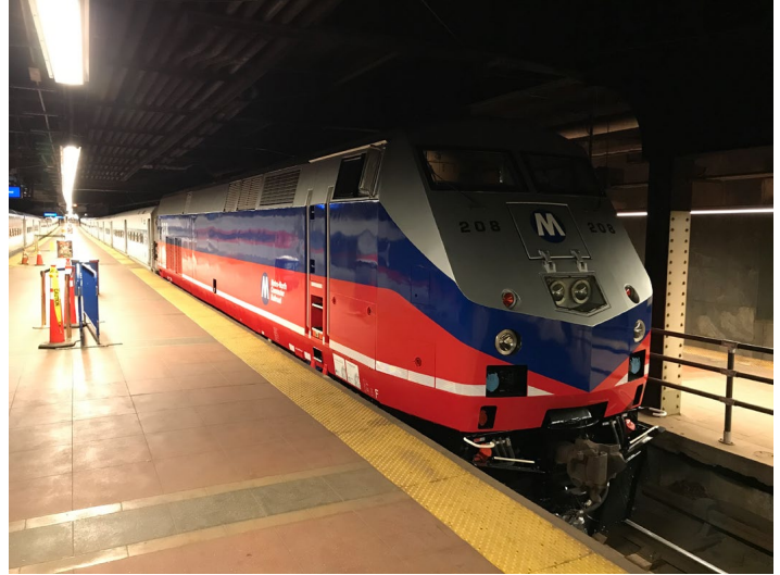
P32AC-DM 208 is seen at Grand Central Terminal on May 23, after its inaugural revenue trip on train #728 from Croton-Harmon. This was taken after the train had been looped so that the locomotive was back on the usual north end. It had come down from Harmon with the locomotive on the south end, contrary to MNR's usual operation. Subutay Musluoglu photo
