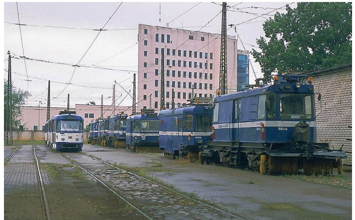
(Above and below) Two scenes of work equipment from further back in the carhouse. No. 88021 is a partly cut-off T3 PCC whose rear was converted for spraying and No. 88006 is a snow sweeper. The lower view shows a further assortment of sweepers with a train of T3s at left.
