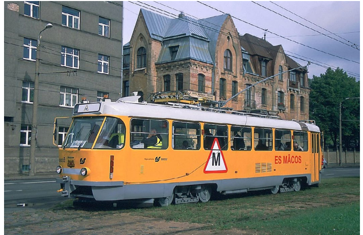
(Above and below) Training car 88032. This beautifully running Tatra T3 PCC was built in 1982 and converted into a training car in 2011. I suspect its conversion into a double-ended unit involved replacing its rear end with the front of another T3. And a pantograph was added to supplement its trolley pole. The upper view shows its formerly blind side with its pole up, while the lower photo shows it operating with a pantograph.
