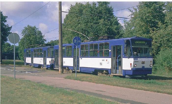
Tatra-built T6 35032, at the point of a two-car train, is in beautiful condition for a 27-year-old vehicle that sees use every day. Riga's roster includes 48 of these angular-looking PCCs.
