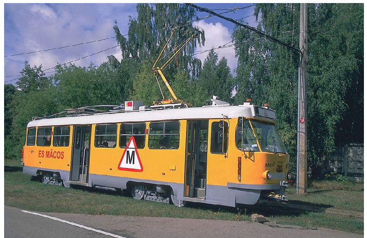
(Above and below) Training car 88032. This beautifully running Tatra T3 PCC was built in 1982 and converted into a training car in 2011. I suspect its conversion into a double-ended unit involved replacing its rear end with the front of another T3. And a pantograph was added to supplement its trolley pole. The upper view shows its formerly blind side with its pole up, while the lower photo shows it operating with a pantograph.
