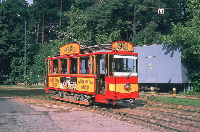
(Above and below) Four-wheeler 1901, emblazoned with tourism slogans in various languages, is a replica, usually used on a fixed route tourist service on Saturdays and Sundays. Built in 1982 by the tramway and Riga carbuilder RVR on an old RVR carbody, it has a great deal of pep and is relatively silent.
