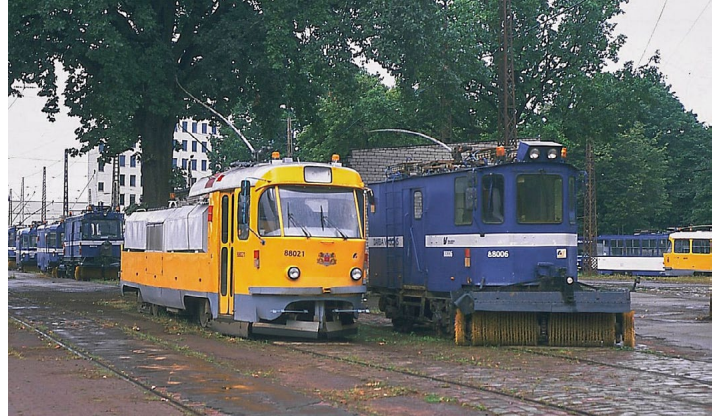
(Above and below) Two scenes of work equipment from further back in the carhouse. No. 88021 is a partly cut-off T3 PCC whose rear was converted for spraying and No. 88006 is a snow sweeper. The lower view shows a further assortment of sweepers with a train of T3s at left.
