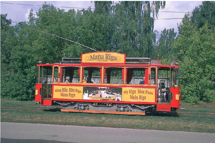
(Above and below) Four-wheeler 1901, emblazoned with tourism slogans in various languages, is a replica, usually used on a fixed route tourist service on Saturdays and Sundays. Built in 1982 by the tramway and Riga carbuilder RVR on an old RVR carbody, it has a great deal of pep and is relatively silent.
