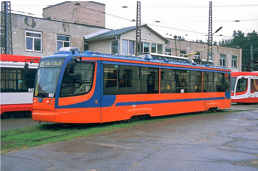
Ust-Katav built KTM-23 No. 007 is in service on route 1 and is shown laying over on the loop at the carhouse. Although it is not apparent, the 2014-built unit is equipped with a low floor in the center.
