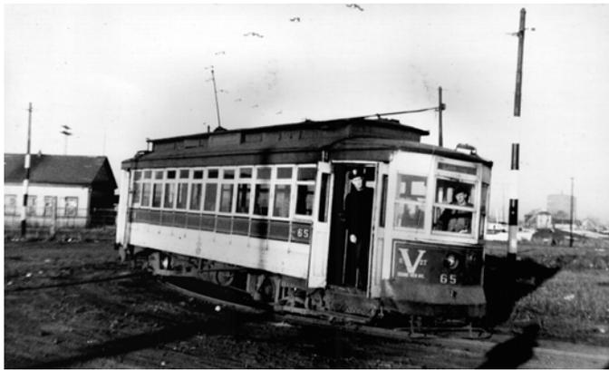
**Car 65 at the Clason Point loop, circa 1946. This is one of the cars speeded up by field shunting.**
