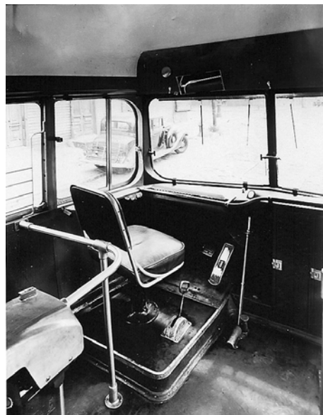
Interior of car 1001, showing the Motorman's seat and controls. Bernard Linder collection
