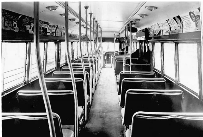
PCC 1001 interior at Ninth Avenue Depot, showing stanchions near every seat on left side. Bernard Linder collection
