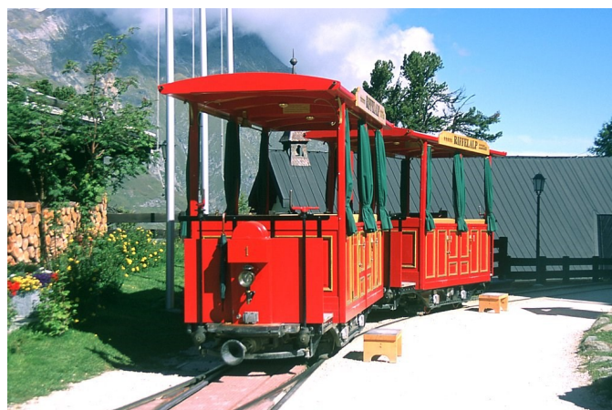
A close-up view of battery car 1 on the 800-millimeter gauge Riffelalp Hotel tramway.
