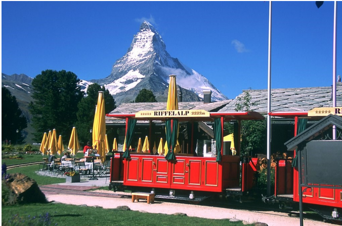
Two views of the Riffelalp Hotel's tramway at its hotel terminal with the Matterhorn looming in the distance. Step boxes aid passengers in boarding and alighting. The track at left leads onto a loop, which is traversed when the train pulls a goods trailer. In normal service the operator just changes ends at the terminal.
