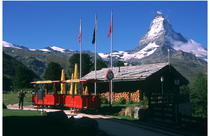
Two views of the Riffelalp Hotel's tramway at its hotel terminal with the Matterhorn looming in the distance. Step boxes aid passengers in boarding and alighting. The track at left leads onto a loop, which is traversed when the train pulls a goods trailer. In normal service the operator just changes ends at the terminal.
