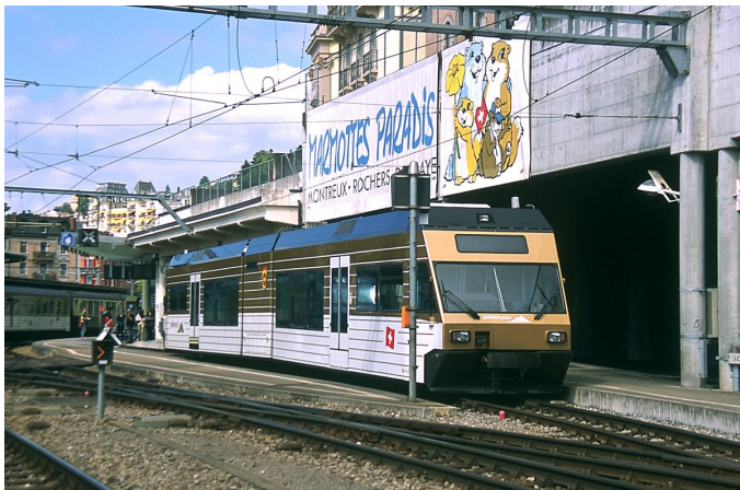
Two views at the Montreux terminal of the MOB/MVR adjacent to the CFF mainline station. A Stadler electric MU car is shown sporting the new color scheme, which recognizes that the line that climbs the mountain is part of the Golden Pass route. In the right view, a similar car in the old livery is shown at left, as well as a locomotive-hauled through train from Montreux to Zweissimmen. The large sign above the Stadler unit advertises MVR's cog railway line that climbs from the lake for over a mile to Rochers-de-Naye, a resort area at an altitude of over 6,400 feet, where there is lots of winter skiing and other activities (see http://www.goldenpass.ch/en/goldenpass/offer/view?id=12 ).
