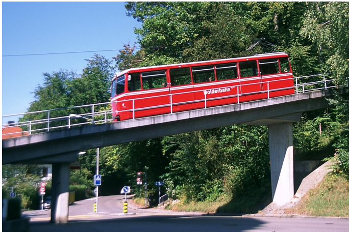
The Dolderbahn was originally a funicular and was not converted to a rack railway until 1972. Its four-wheelers were built at that time by SLM (now Stadler) in Winterthur and contain Brown Boveri electrical equipment for operation from 600-volt d.c. overhead (the same as Zurich's streetcars). The left view is just beyond the Waldhaus station near the outer end of the line, while the right photo shows an out-bound car just leaving the Titlisstr station before reaching the line's passing siding.
