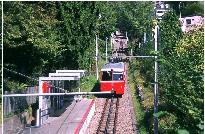
The Dolderbahn was originally a funicular and was not converted to a rack railway until 1972. Its four-wheelers were built at that time by SLM (now Stadler) in Winterthur and contain Brown Boveri electrical equipment for operation from 600-volt d.c. overhead (the same as Zurich's streetcars). The left view is just beyond the Waldhaus station near the outer end of the line, while the right photo shows an out-bound car just leaving the Titlisstr station before reaching the line's passing siding.
