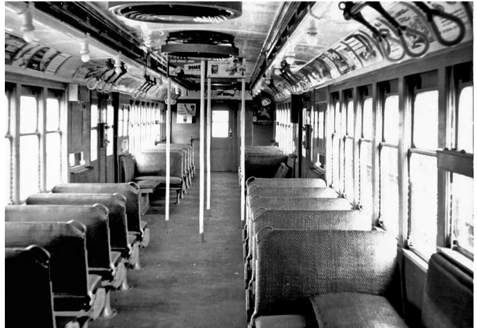
Interior of NYCT 2902 (ex-SIR) in Coney Island Yard, March 3, 1955. Note Axiflow fans that were installed by NYCT, Bernard Linder photograph
