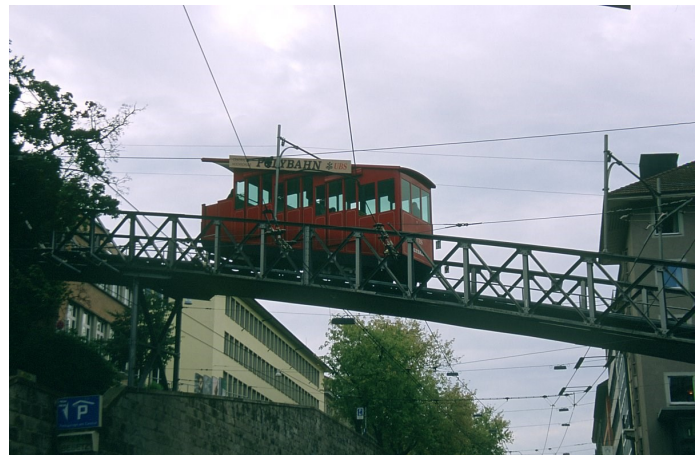
The Dolderbahn was originally a funicular and was not converted to a rack railway until 1972. Its four-wheelers were built at that time by SLM (now Stadler) in Winterthur and contain Brown Boveri electrical equipment for operation from 600-volt d.c. overhead (the same as Zurich's streetcars). The left view is just beyond the Waldhaus station near the outer end of the line, while the right photo shows an out-bound car just leaving the Titlisstr station before reaching the line's passing siding.
