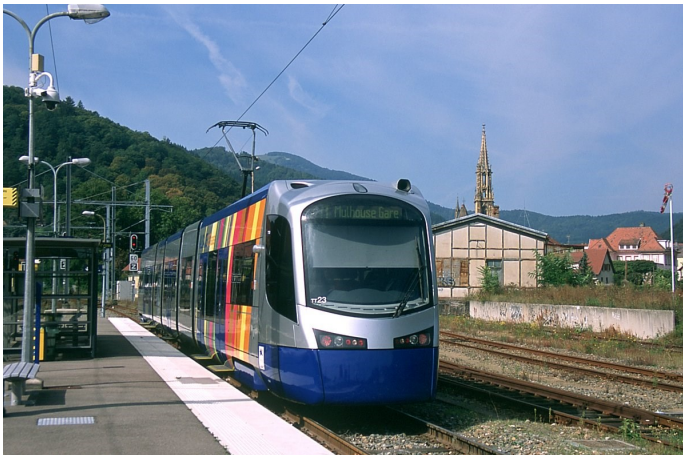
A Siemens Avanto tram-train at the Thann Gare station. Note the step that slides out from the body of these 70 percent low-floor cars at each door.
