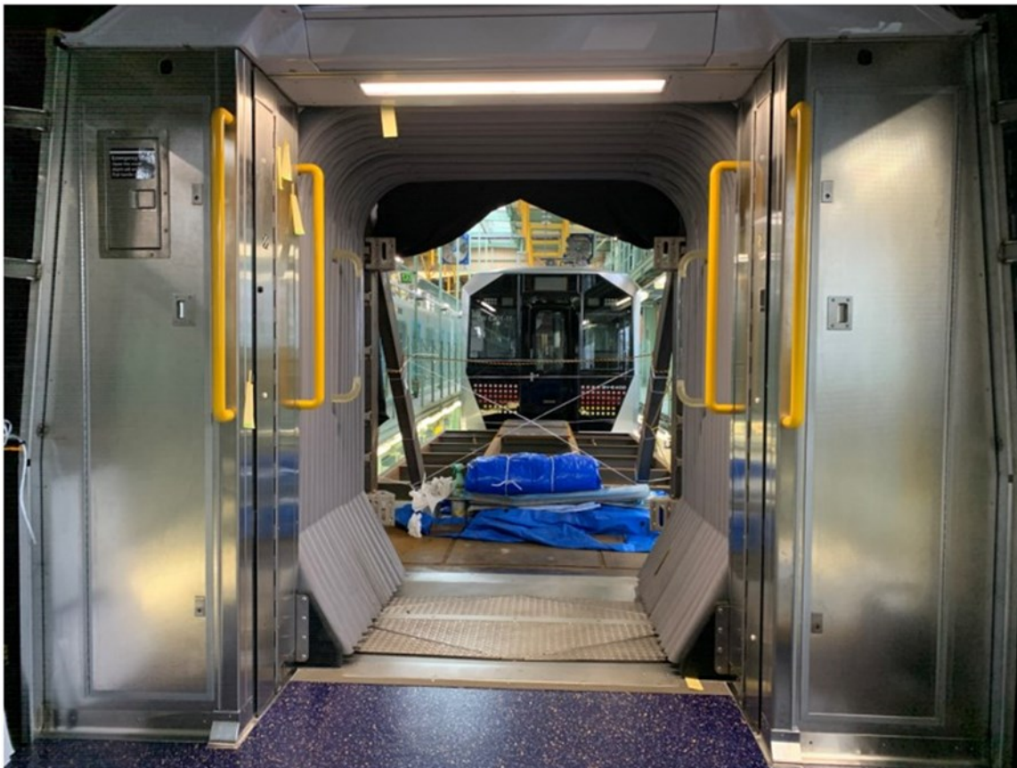
A view of the open gangway that will be between cars without operating cabs.
