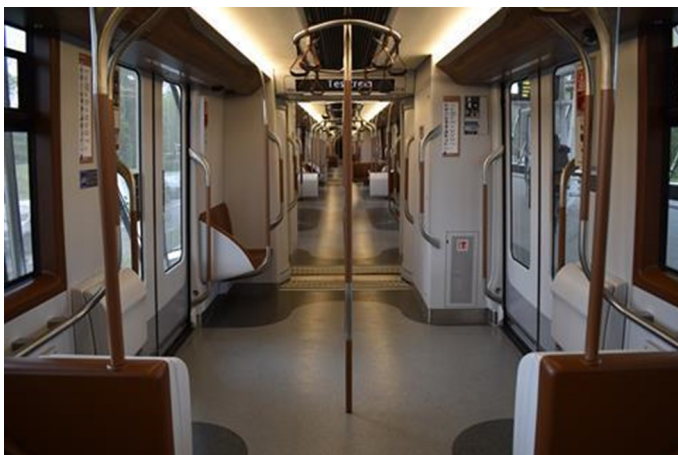
The M7 sets provide a mix of transverse and longitudinal seating as well as open gangways.
