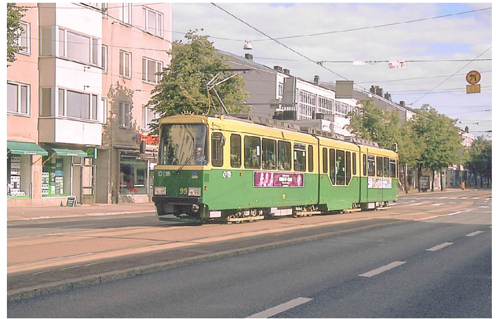
(Above and below) Two views of Valmet-built cars along Mannerheimintie, a major arterial that runs from the northwest portion of Helsinki to downtown. These cars were constructed from 1983 to 1987 as two-section articulated units, but had low-floor center sections added between 2009 and 2011.
