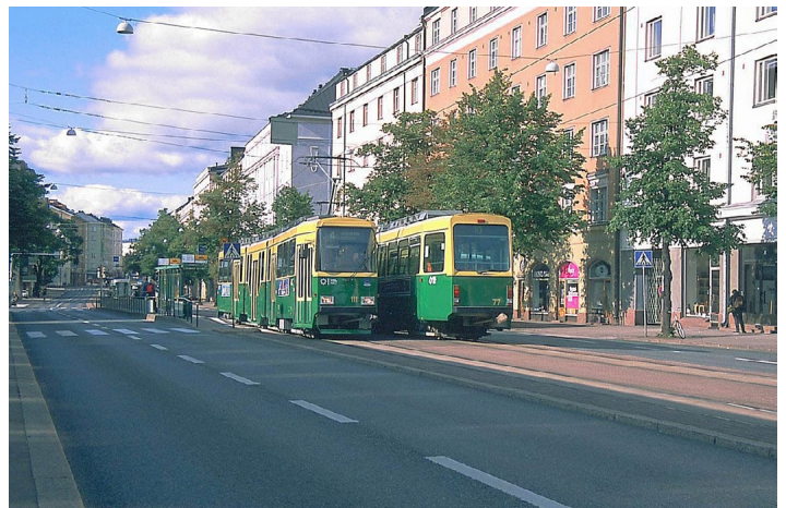
(Above and below) Two views of Valmet-built cars along Mannerheimintie, a major arterial that runs from the northwest portion of Helsinki to downtown. These cars were constructed from 1983 to 1987 as two-section articulated units, but had low-floor center sections added between 2009 and 2011.
