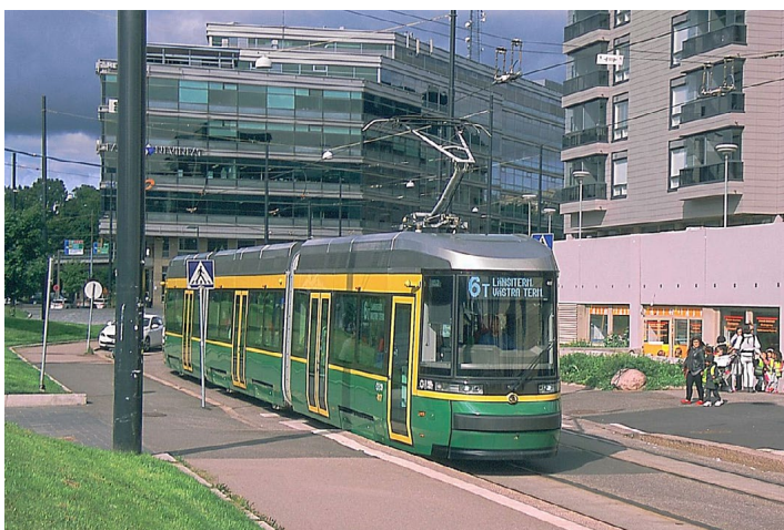
Helsinki's newest cars are 44 three-section 100-percent low-floor Škoda ForCity Smart units built in the past three years. No. 417 is shown approaching its Hietalahti terminal on Ruopohlahdenranta in front of our hotel.
