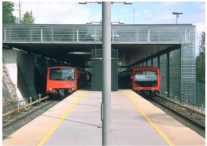
The 300s (right) are four-car sets, but the platforms can fit six-car trains. Since I didn't ride in the rush hour I don't know whether six-car trains were being operated with other equipment later in the day.
