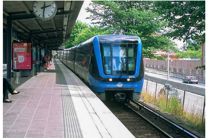
(Above and below) Alvik station is the transfer point between the T-bana's Green Line and both the Nockebybanan and Tvarbanan light rail routes. The Metro runs left-handed, as shown in these views of trains of Vagn 2000 (C20) cars. The lower photo shows the rear of an inbound subway train across the platform from an inbound Nockebybanan tram, which has deposited its passengers and is about to navigate the scissors crossover; it will pick up new riders at the opposite platform. These route 12 trams use a second crossover beyond the station to achieve right-hand operation (photo to be shown in Part XXXI), a complication unnecessary before the 1967 changeover in the rules of the road. There are 270 of these Movia C20 cars (90 three-car sets) in service on the T-bana, which were built in 1997-2004 by the Swedish subsidiary of Adtranz (now Bombardier). Older traditional cars from the 1970s and 80s also provide service (mostly in rush hours), and will be gradually replaced by Bombardier cars (C30s) now under construction. Both photos were taken in 2016.
