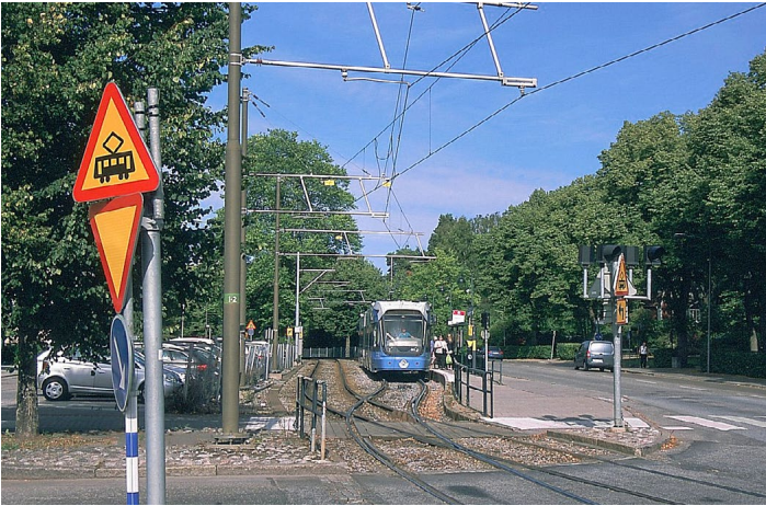
Outbound Flexity Swift car 411 stops at the Alléparken station, just before crossing the inbound track (whose platform is behind the photographer). The crossover was constructed in 1967 when the Nockebybanan was converted from left-hand to right-hand running, except for its access to the across-the-platform transfer point with the T-bana's Green Line at Alvik station.
