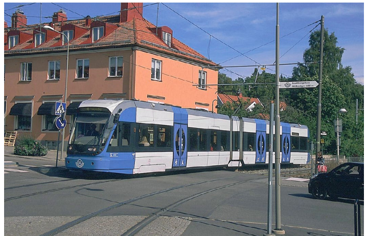
(Above and below) Two views of the Nockebybanan at its Älstenstgatan stop, about halfway along the route. Outbound car 427 is a three-section low-floor Flexity Swift (A32) unit built by Bombardier in 2009.
