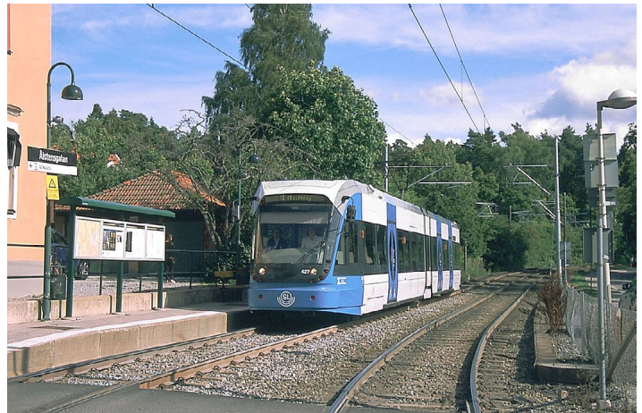
(Above and below) Two views of the Nockebybanan at its Älstenstgatan stop, about halfway along the route. Outbound car 427 is a three-section low-floor Flexity Swift (A32) unit built by Bombardier in 2009.
