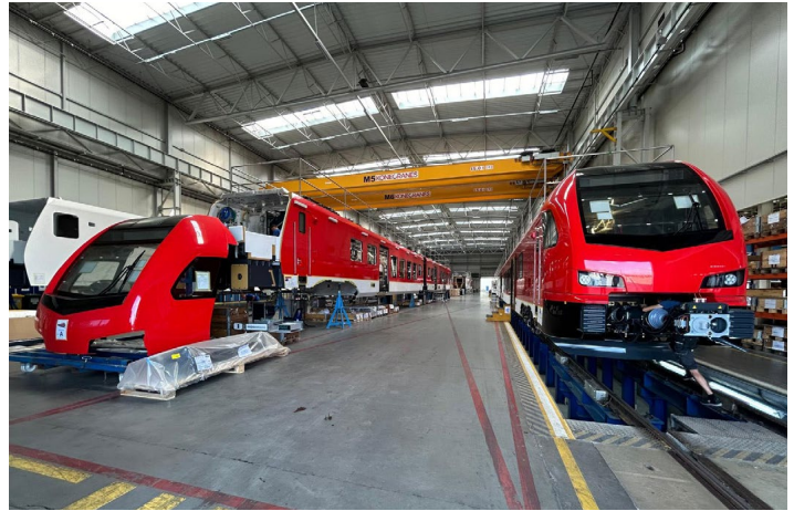
The new Class ETR 814 FLIRT EMUs under construction at the Stadler factory in Siedlce, Poland. Silvia Savoye photo via Wikipedia
