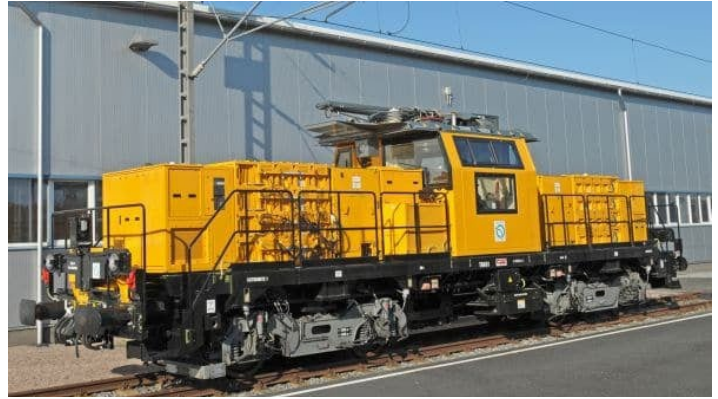
The CAF-built battery locomotive for use on Paris RATP's RER lines, at the Velim testing grounds in the Czech Republic. Quintus Vosman photo
