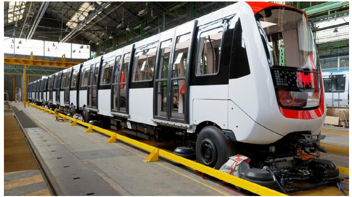
Lille metro trainset being assembled at Alstom's Valenciennes-Petite Foret site. Samuel Dhote/Alstom photo
