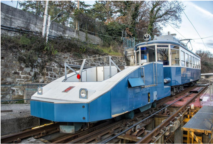
One of the tractors, built in 2005, with double-truck motor No. 405 (Officine Meccaniche Stanga, 1935) at the upper station of the funicular section of the line, Vetta Scorcola. These newest tractors have no cab, greatly improving visibility for the tram drivers, who now control them. Toma Bacic photo
