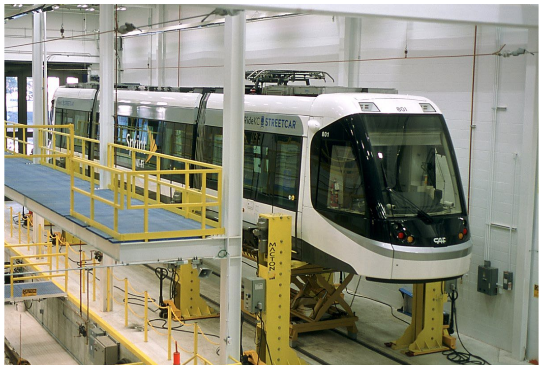
(Below) Double-ended CAF-built three-section articulated low-floor car 801 is shown undergoing maintenance on one of the hoists in the Streetcar Authority’s Singleton shop.
