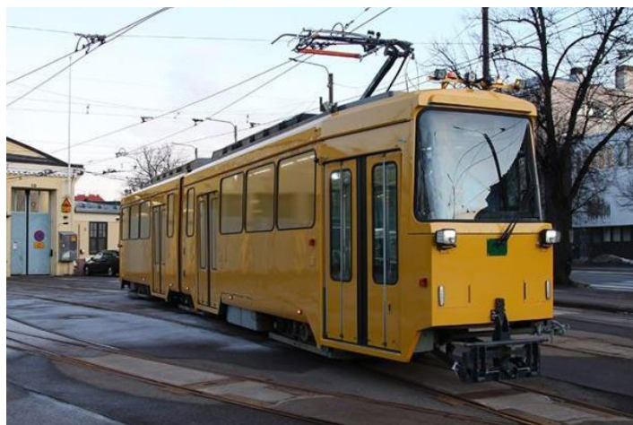
The catenary de-icer had been a Valmet MLNRV2. It was originally a class Nr II. When modernized between 1996 and 2005, it was redesignated as Nr II+ class. It had received a low-floor middle section between 2006 and 2011. Helsinki City Transport (HKL) photo
