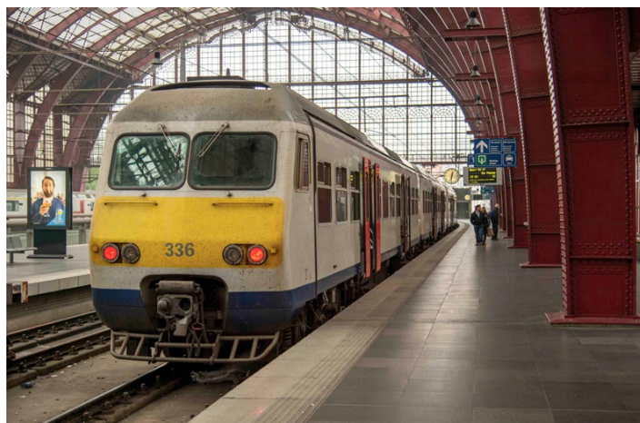
Typical of the older type of EMUs to be replaced under this new order is Class AM 80 No. 336 (La Brugeoise et Nivelles, 1980-83), seen at Antwerpen-Centraal on May 2, 2019. Jeff Erlitz photo
