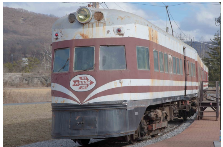
Liberty Liner “Independence Hall” is one of two former articulated high-speed interurban “Electroliners” built by the St. Louis Car Company in 1941 for the Chicago, North Shore & Milwaukee. Designed to operate on the Chicago “L”, they were sold to the Philadelphia Suburban Transportation Company’s Red Arrow system in 1963. SEPTA sold the interurban to the museum in 1981.
