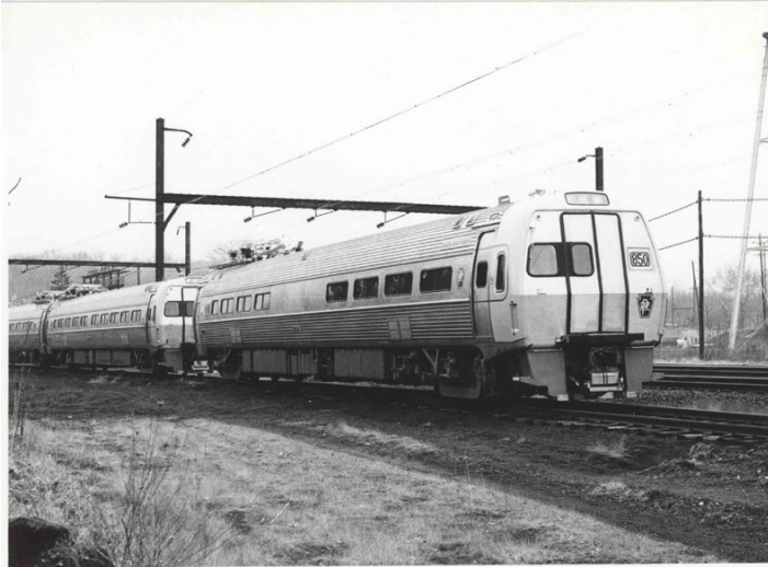
Metroliner production snack bar coach car #850 at Jenkintown, Pennsylvania shortly after delivery by Budd in 1967. This was the first car equipped with G.E. propulsion (versus Westinghouse) delivered. Date and photographer unknown. ERA Collection.
