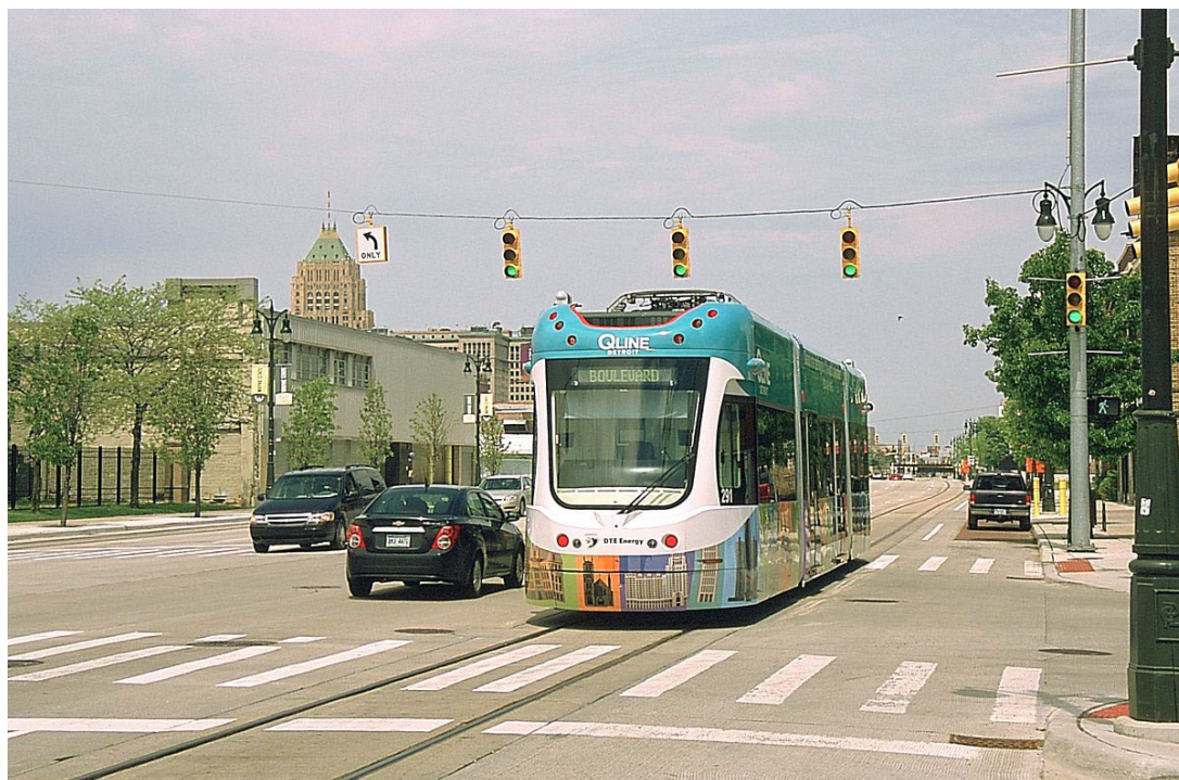
(Left) The rear of a Grand Boulevard-bound car is shown crossing Palmer, just slightly south of the freeway. This view illustrates one of the sections of the line where the tracks have been placed to leave room for parallel parking along wide Woodward Avenue. However, this can result in delays, especially when automobiles are not parked close enough to the sidewalk, but fortunately there is much more leeway here than there is in Washington, D. C., where narrow H Street leaves virtually no room for error. I should point out that I found it a bit dangerous to jaywalk into the center of Woodward Avenue to take photos like the one with the billboard.
