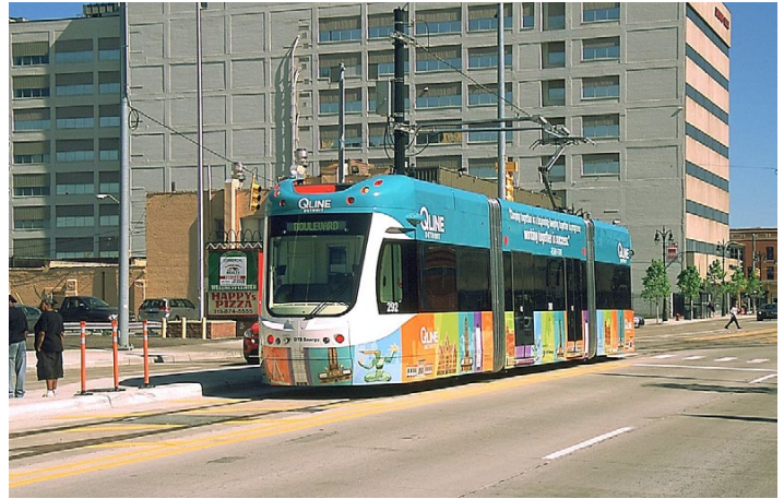
(Above and below) This Brookville Liberty streetcar had to be positioned carefully so its pantograph could be raised to allow its batteries to be charged from 750-volt DC overhead. The car will be battery-propelled from this point southward until it reaches the Ferry Street station and enters upon a stretch containing poles and wire. It is said that the use of ugly overhead on streetcar and light rail lines can destroy the quality of the views in the area. The upper photo shows the tracks turning right (eastward) into the Penske Tech Center, where rolling stock is maintained and stored overnight. This approach to charging batteries is also used on the Dallas Streetcar but is accomplished during the period while revenue cars lay over in the terminal station. The operator, M-1 Rail, states that the tech center is the only wireless facility in the U.S. One more track branches off one of the main tracks inside, to give a three-track facility.
