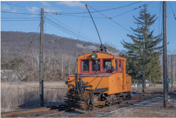
Scranton Transit No. 107 is a double-ended snow sweeper built in-house as number No. 99 by the Chicago and Joliet Electric Railway in 1910 and sold to Scranton Transit in 1933 after the C&JE abandoned streetcar service. When Scranton closed in 1954 No. 107 was in the collection of various museums until it ended up at Rockhill in 1973.
