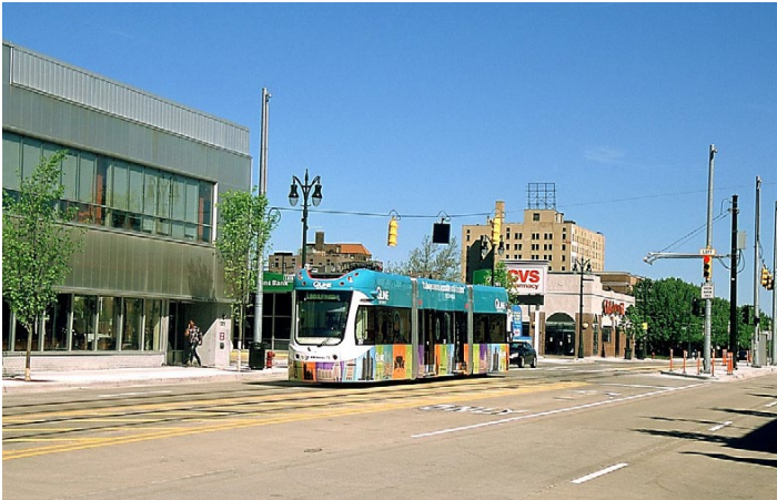
This Brookville Liberty car is shown returning to the Grand Boulevard terminal to begin a southbound run after having its batteries charged in the area adjacent to the traffic signals at right. The double-track merges into one before fanning out again to enter the carhouse. Close-up views are on the right.
