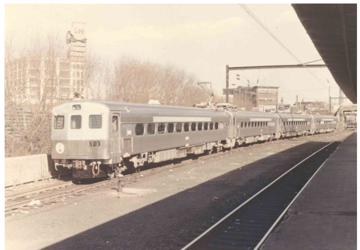
Color view of high-speed test car T-3 leading the four-car test train. Visible on the letterboard along the side of the car is the text "US DEPARTMENT OF TRANSPORTATION TEST CAR." The Lee clothing factory in the background means that this is Trenton, New Jersey. Date and photographer unknown. ERA Collection.
