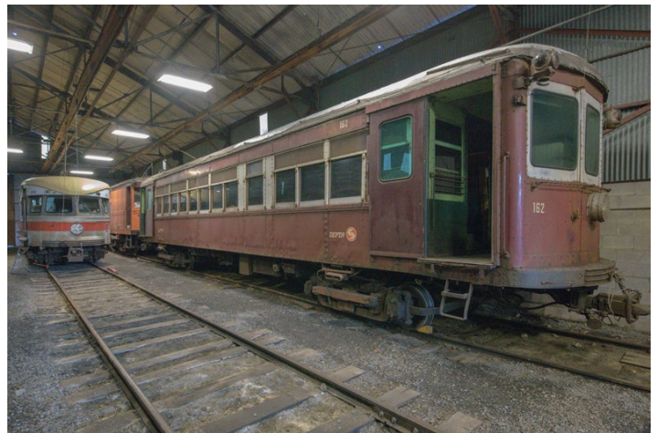
SEPTA No. 162 was built in 1927 by J. G. Brill Company for the Philadelphia & Western Railroad. Following rebuilding in 1931 the car was mostly assigned to the Strafford Branch of the P&W until abandonment of this branch in 1956, when it was reassigned to other lines, like the Norristown line. The Rockhill Museum worked to restore the car to operation, and it debuted at Winterfest. There is still cosmetic work to be done but it was great to see the car operate again.
