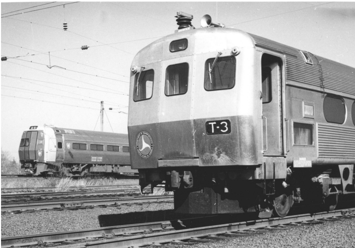
Pioneer III high speed test car T-3 with production Metroliner coach car #803 in the background. This view shows the detail of the high-speed end cap and some of the exterior writing for the test equipment. Location, date and photographer unknown. ERA collection.
