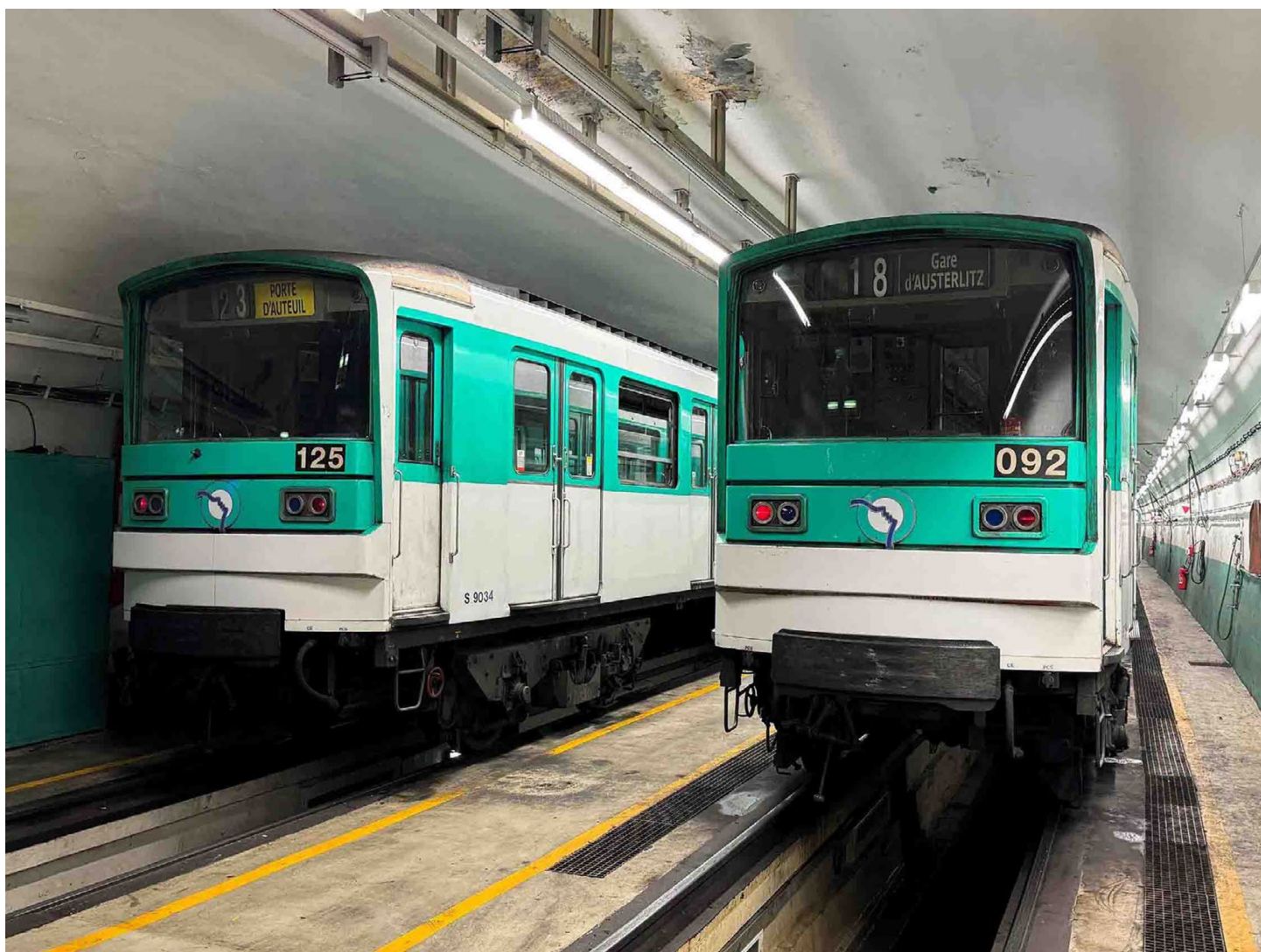
Two trains of MF67 stock are seen at Line 10's underground depot at Auteuil on September 20, 2024. On the left is MF67CX trainset No. 125 (Alsthom-Groupe Brissonneau/SFB-Societe Franco Belge, 1974), composed of S.9034-N.11223-NA.12125-N.11071-S.9033. On the right is MF67C2 trainset No. 092 (Brissonneau et Lotz, 1971), composed of S.9158-N.11175-NA.12092-N.11187-S.9017. Subutay Musluoglu photo
