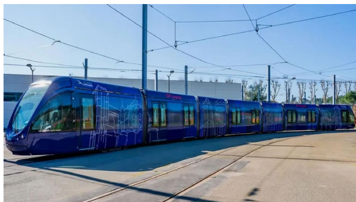
The first of the Citadis 302 trams that was extended from five to seven sections. SETRAM photo
