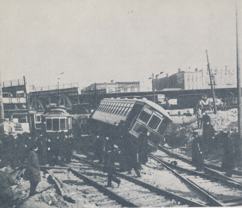
Motorman Kiernan's brakes failed on car 31 in December, 1914 on the downgrade and this was the end result.
