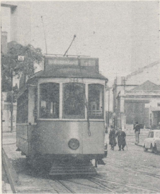
A Lisbon double-truck tram is about to take the switch to the Amara car-barn. This type tram originally had a deck roof. --Bruce Russell
